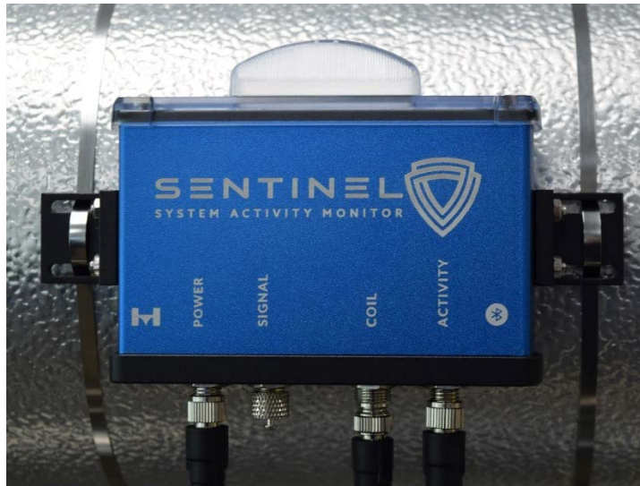
Figure 5. Installation of the analyzer on a pipe.
