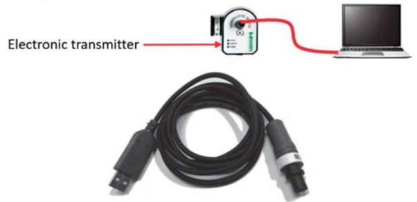
7. Open the Hansen tool and press Start scanning to initiate connection to the sensor. 3 LEDs will display around the M12 connector. Green, red and yellow LEDs will flash when the communication is active.
