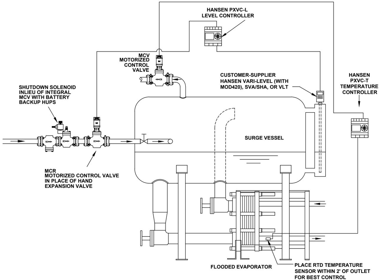
**TYPICAL LIQUID INJECTION COOLING FOR SCREW COMPRESSOR APPLICATION**
