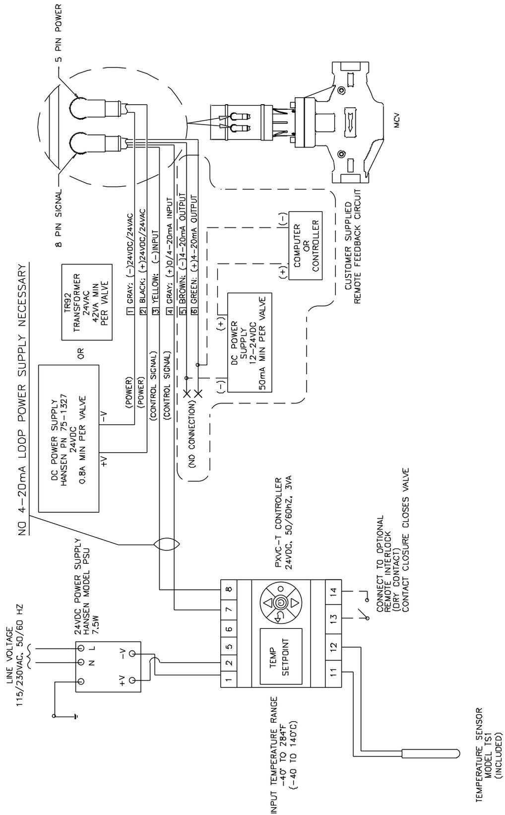
PXVC-L (LIQUID LEVEL) WIRING DIAGRAM, 115V/230V
