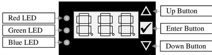
All LEDs will be on for couple seconds on power-up. After that the Red and Blue LED should not turn on. The Green LED indicates valve is in manual mode (H.02). To enter and navigate the menu, follow the steps below:
