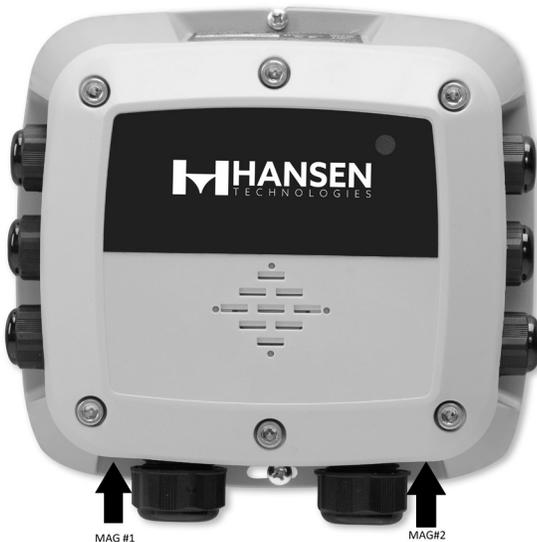
User interaction with the gas detector is accomplished through the use of two magnetic switches located on the bottom of each unit. To actuate a magnetic switch (referred to as MAG#1 or MAG#2), apply the supplied magnetic wand) to the relevant switch location as indicated below:
