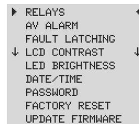
From the RELAY menu, each of the three relays can be configured for either normal or failsafe operation. The default is normal, meaning normally open contacts will close with the event corresponding the relay designation. If fail safe is selected the relay will be normally energized and will be de-energized with the relays designated event or a power failure.
